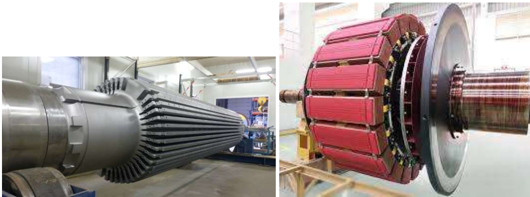
Slika 1.4.1 Izgled turbogeneratora (lijevo) [ https://hwr.bhel.com/bhelweb/portfolio_details_tg.jsp ] i hidrogeneratora (desno) [ https://voith.com/corp_en/Voith_Small_Hydro_Generator.pdf ].
